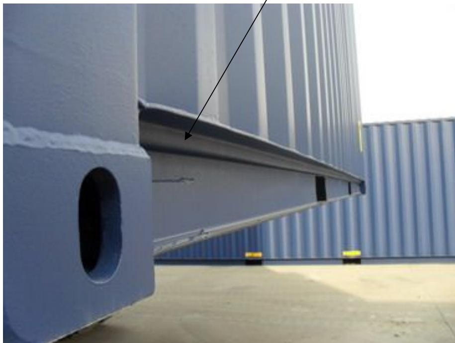
Bottom Side Rail (Double “Z” Section)
