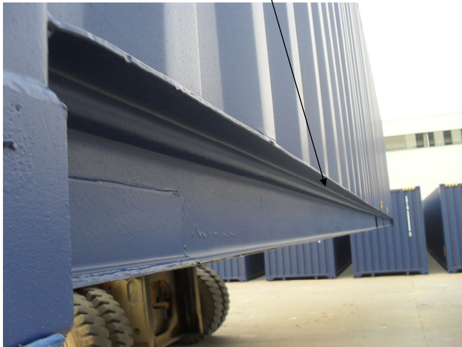
Bottom Side Rail (Double “Z” Section)
