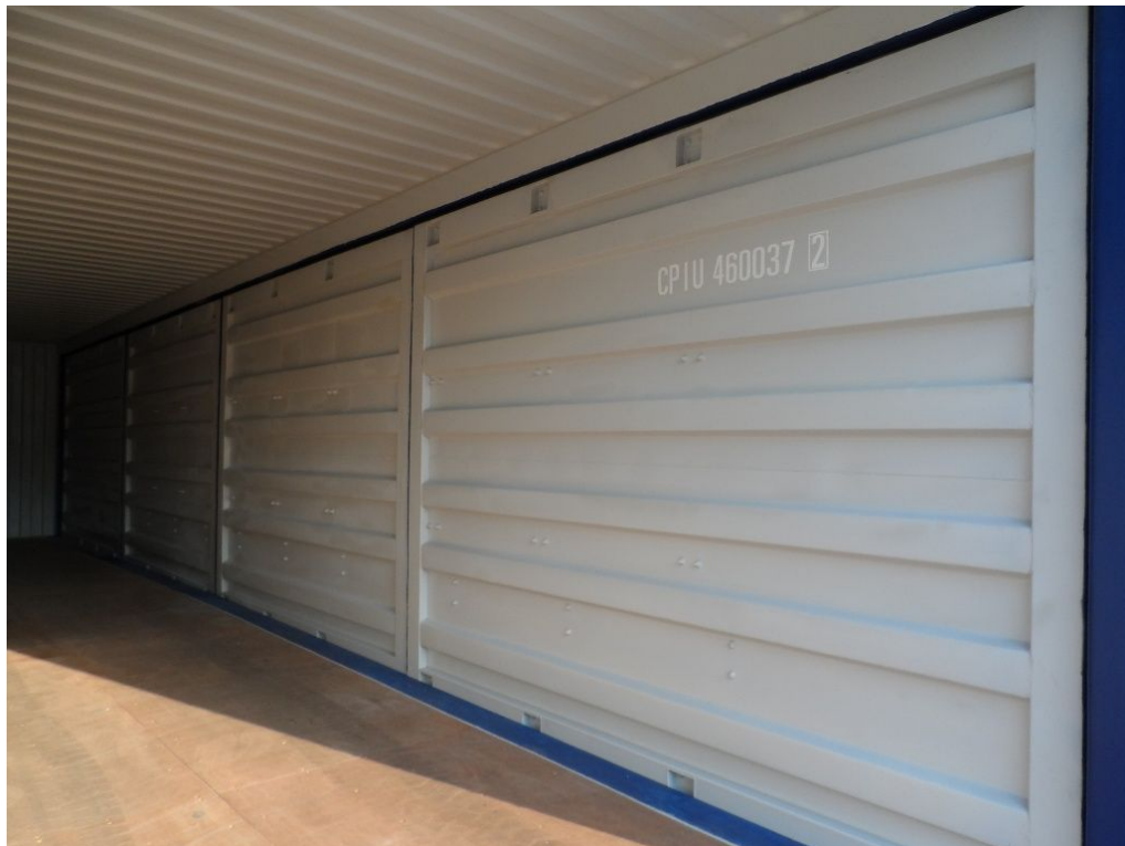
Internal Right Side Wall Without Lashing Rings
