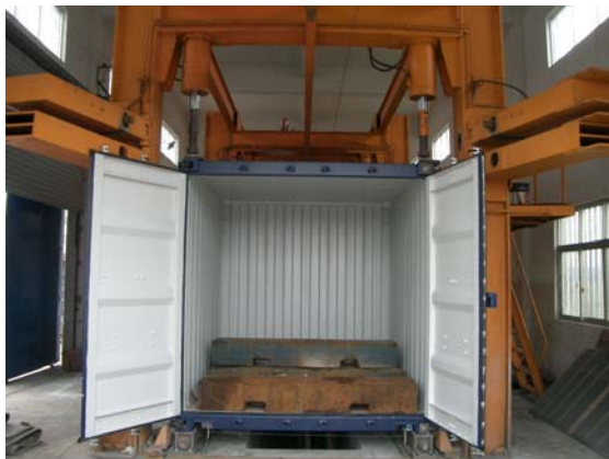
Connectors Strength Test (payload:10T Per 10') Lifting Test From Top/Bottom Corner Post
