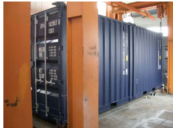
Connectors Strength Test (payload:10T Per 10') Lifting Test From Top/Bottom Corner Post
